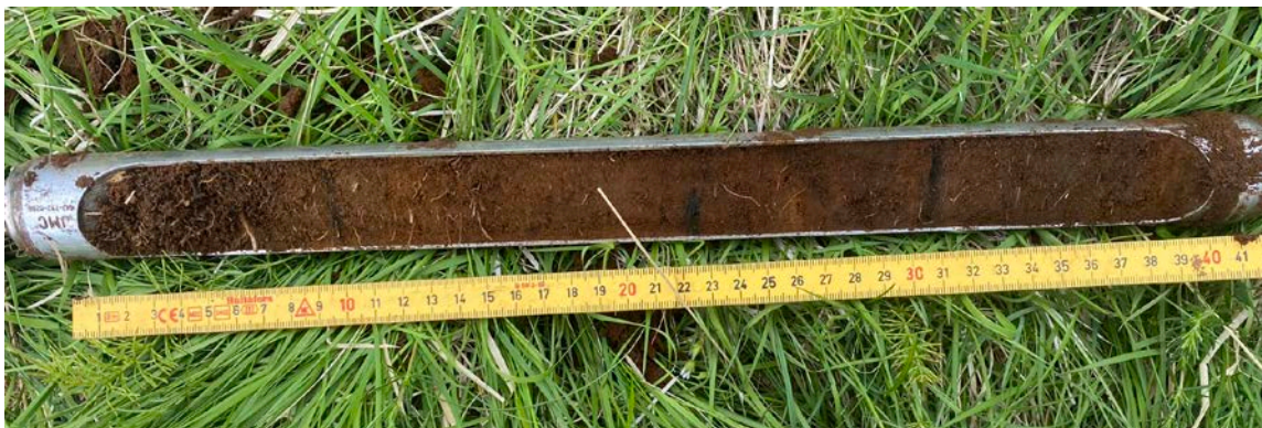
Figure 70: Layers in core 11_14. Thin line of a possible black tephra 10 cm down. Turf deposit with grey tephra and a line of grey tephra (possibly H-1300), possibly in situ. No samples were taken from the core.
