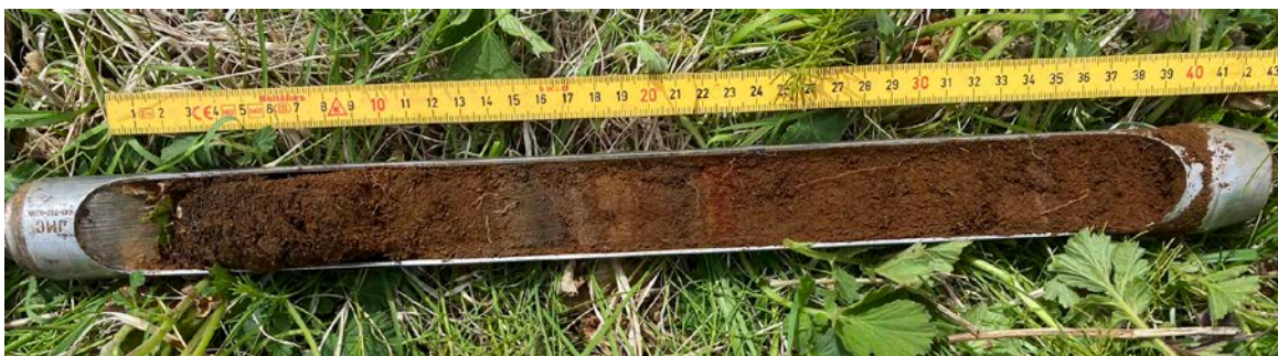
Figure 71: Layers in core 11_19. Turf deposit with grey tephra (possibly H-1300) and light brown, yellowish brown, and red lines. Very thin white organic line 34 cm down.
